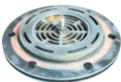
3rd stage air-cooled valve after 2,500 hours
