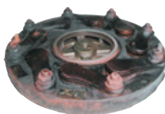
2nd stage water-cooled valve after 800 hours
